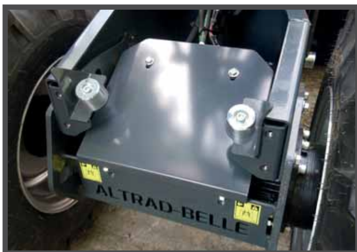
ROBUST STEEL, FRONT MATERIAL INGRESS GUARD PREVENTS DAMAGE TO HYDRAULIC CIRCUIT
