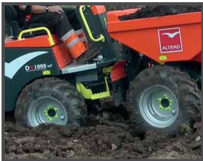
HIGH-QUALITY, ALL-TERRAIN TYRES WITH VALVE PROTECT GUARD & WHEEL NUT INDICATORS
